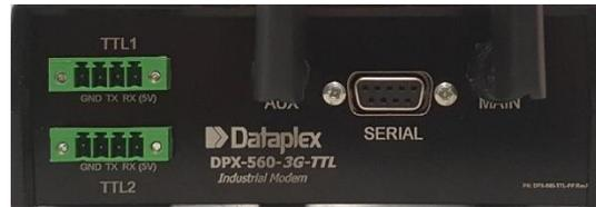
The Dataplex 3G M2M Router (DPX-560) offers an easily integrated solution that is simple to manage, configure and customise. Designed to enable diverse M2M applications, the DPX-560 connects to 3G networks, comes equipped with GPS and multipurpose interfaces including I/O, Serial and Ethernet (USB is optional). TTL option is also available, where the modem uses up to two TTL interfaces to communicate to TTL aware devices.
